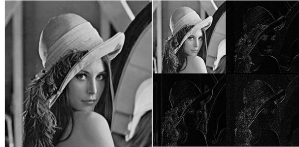
Figure 1.3 Right one shows the wavelet decomposition of the left picture. It uses 1 level Db4 wavelet decomposition in the Matlab. The image size is 512x512
